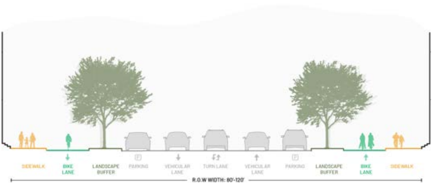
Figure SP-13 Illustrative Cross Section for Local Bike + Car Street
