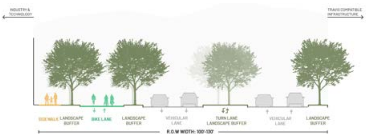
Figure SP-16: Illustrative Cross Section for Collector 1 (Access Boulevard)
